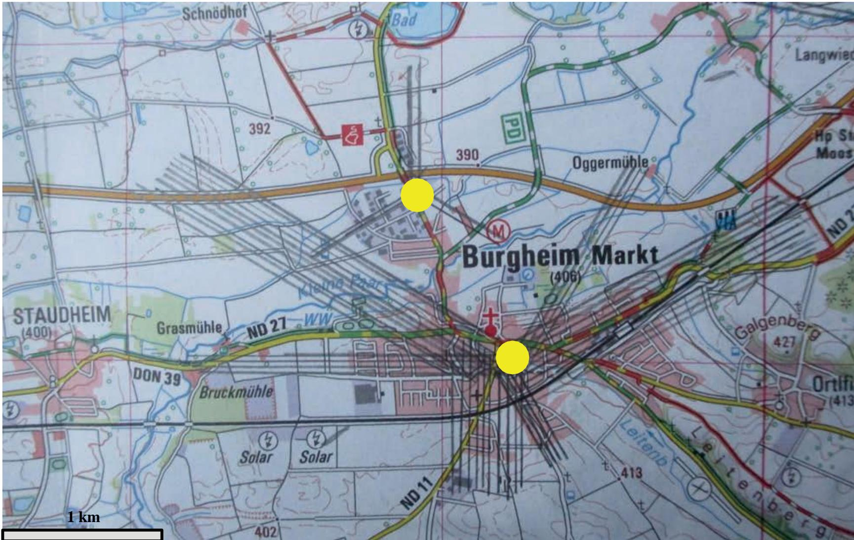
Section UK 50-34, Bavarian State Agency for Digitization, High-Speed Internet and Surveying (LDBV). Added: locations of mobile phone base stations with the main beam directions of the sector antennas
